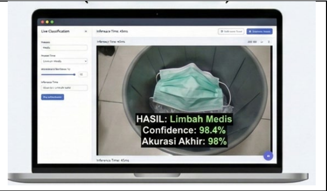
Figure 2. Real-time On-device Classification Output Showing Predicted Medical Waste Category and Confidence Score Using the TinyML-based Sensor Fusion System
