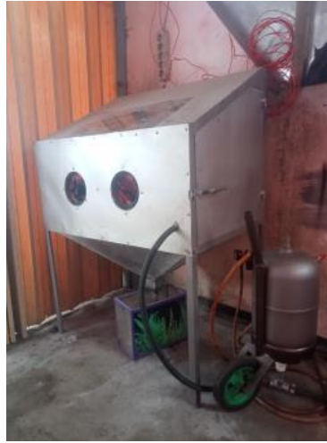
Figure 4. Fabricated portable sandblasting prototype
