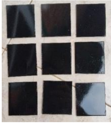
Figure 2. Aluminum test specimens (50 × 50 × 2 mm) coated with commercial paint prior to blasting
