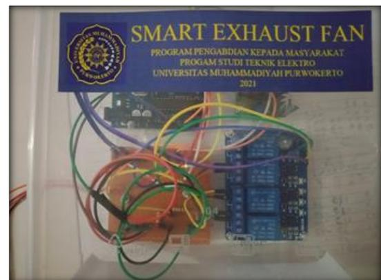
Gambar 3. Rangkaian pengendali smart exhaust fan
