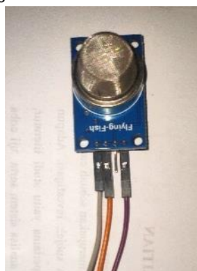
Figure 10. MQ2 sensor test
