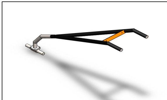
Figure 2. 3D Weed weeding machine frame
