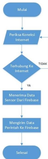
Gambar 9. Flowchart Sistem Smartphone
