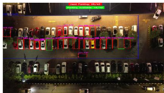
Fig. 7 YOLOv8 detection performance at night
