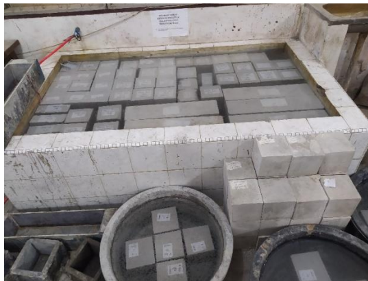
Gambar 2. Benda uji beton – pasir lahar dingin
