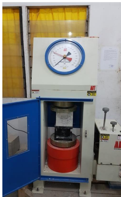
Gambar 2. Benda uji beton – pasir lahar dingin
