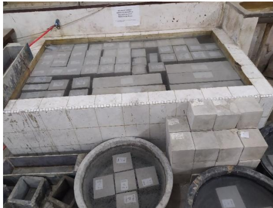
Gambar 2. Benda uji beton – pasir lahar dingin
