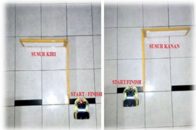
Gambar 8. Arena pengujian robot wall follower
