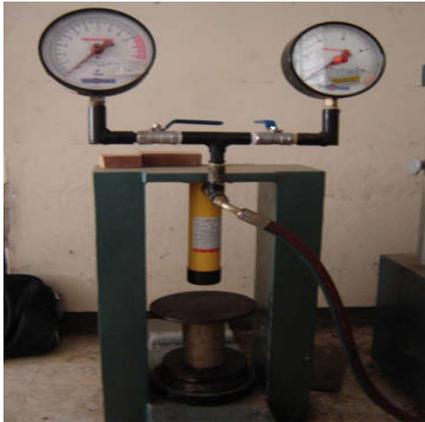
Gambar 2. Flexural Testing Machine
