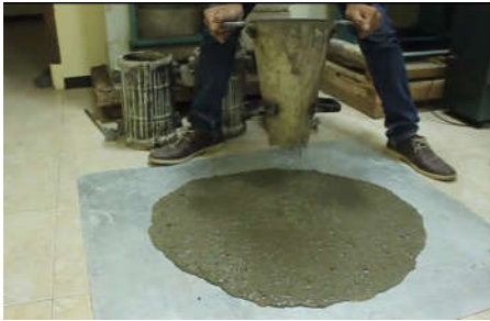
Gambar 3. Proses uji slump
