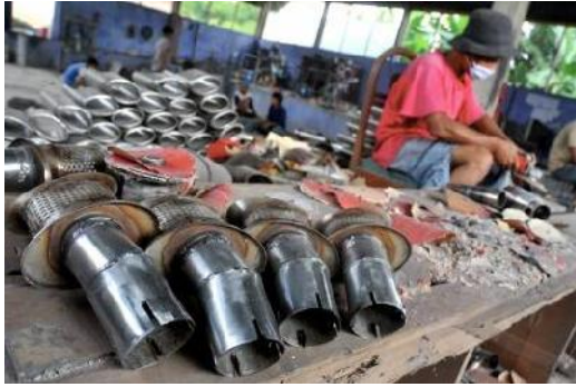
Figure 1. Example of mufflers production site with simple or handmade manufacturing processes
