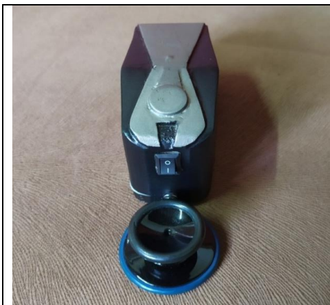
Figure 1. Design of the Electronic Stethoscope
